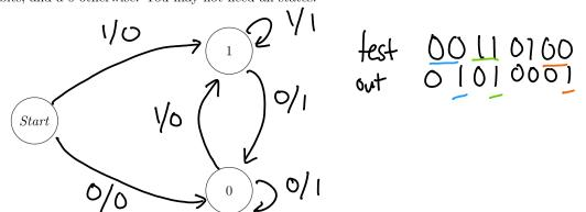
$\boxed{3.3}$  Write an FSM that will output a 1 if it recognizes the regex pattern  $\{10+1\}$ .
